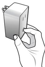
3. Plug the PD-100 back into the AC outlet with the button pressed
